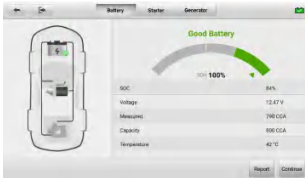
Figure 6-7 Sample Battery Test Results Screen
