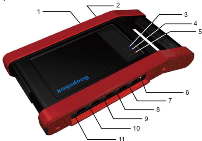
Figure 2-3 Scopebox structure view
