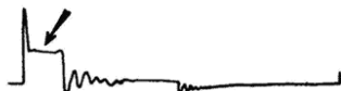
Spark plug gap is too large or mixture gas is too lean
