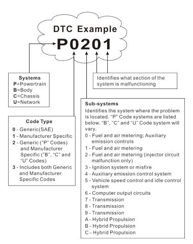
P0201 - Injector circuit malfunction, Cylinder 1
