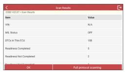
Note: A PROTOCOL is a set of rules and procedures for regulating data transmission between computers, and between testing equipment and computers. Now five different types of protocols (ISO 9141, Keyword 2000, J1850 PWM, J1850 VPW and CAN) are in use by vehicle manufacturers.
